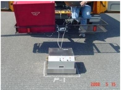
Figure 8 Circular Track Meter (CTMeter)
